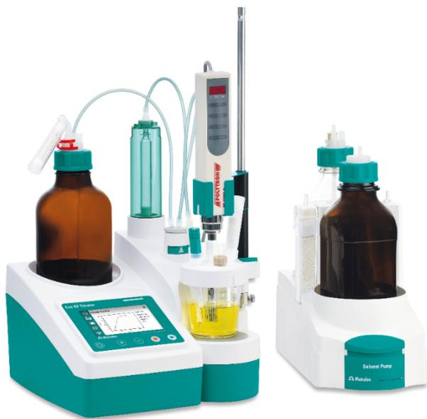
**Figure 1.** Eco KF Titrator equipped with a Polytron, a Solvent Pump, and a double Pt-wire electrode for volumetric Karl-Fischer titration.
